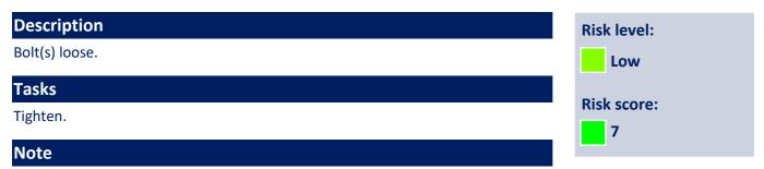
Bridge connectors are slightly loose to platforms. Multiple barrier, hand holds and climbing ramp bolts are slightly loose. Tighten all loose fixings.
